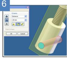
Your teacher shall show you how to apply a workplane. SKETCH a circle diameter 4 on this plane, and extrude a hole all the way through.
